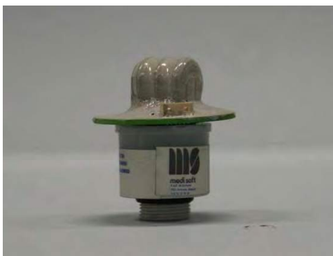
Cell replacement for NO analyzer
